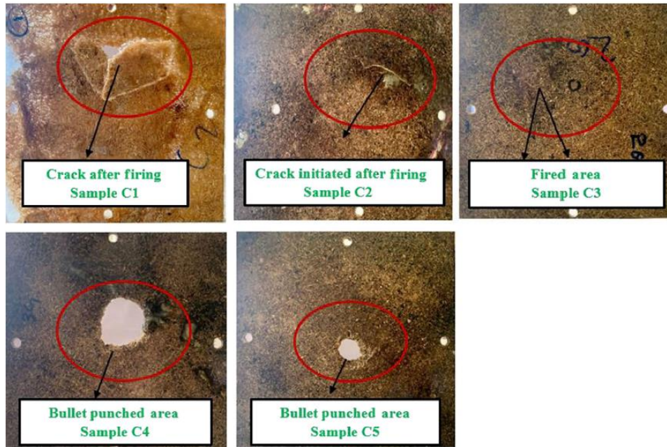
Ballistic impact tested samples of various composites
